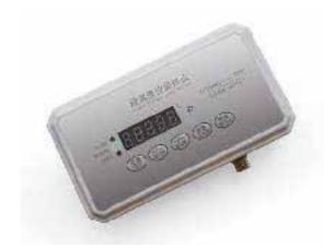
Cryomonitor 1000 liquid level monitor (left)
